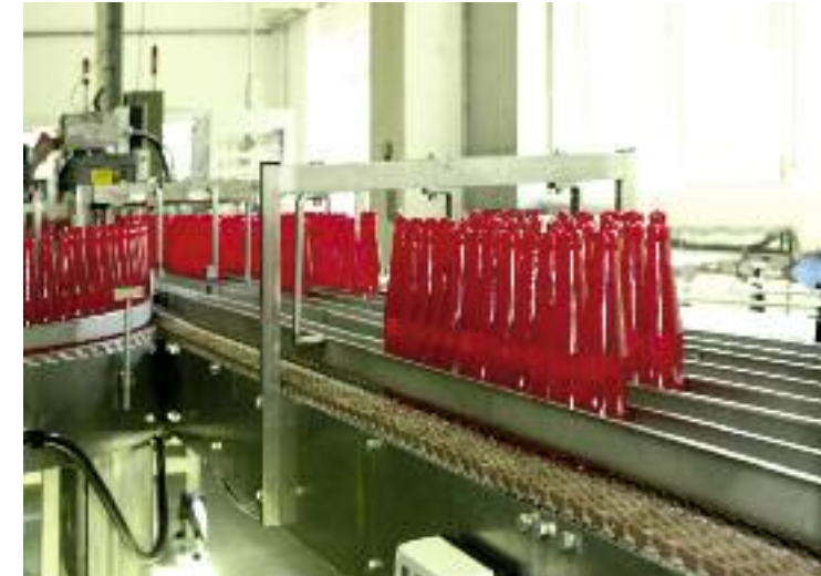
The specially designed filling system takes over filling and sealing in one operating cycle
